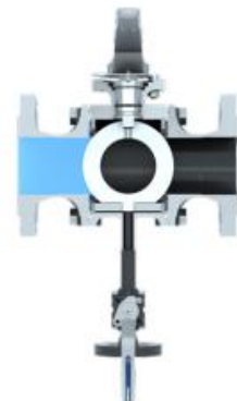
KHA ball valve completely closed with opened drain cock. Dead space and ball completely emptied.
