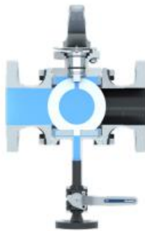
KHA ball valve completely closed, dead space and ball filled with medium
