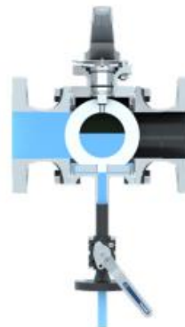
Opening of the drain cock. Complete drainage of the dead space and inner space
